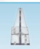
Available In Clear Or Color-Matched To Any Standard Roofing Color Manufactured from clear UV-stabilized Lexan-grade polycarbonate material, or available in a color that is injected throughout the product and can be matched to any standard roof panel. The Sno Gem Junior offers a 12.5 square inch bonding surface and is recommended on panels with intermediate ribs. Apply adhesive using 3M VHB Tape, tube adhesive, or a mechanical fastening application.
